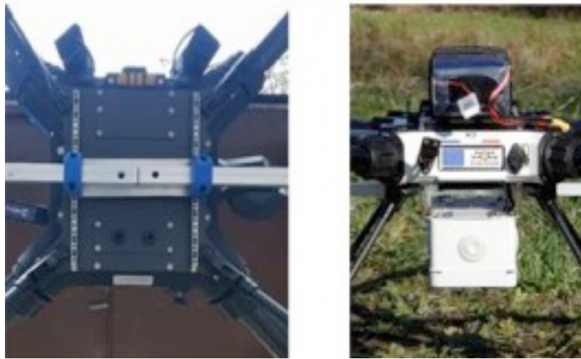
Figure 6: mounting configuration of the antennas and the dummy radar.
