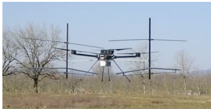
Figure 7: In-flight UAV with attached antennas and dummy payload.
