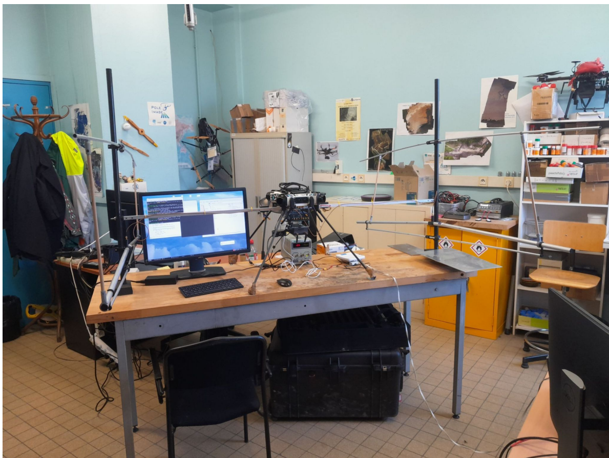
3 Figure 5: Test of the radar in the laboratory with the drone in “off” position. The radar is installed on board the drone. The GPR antennas are visible on both sides of the drone. The computer is connected to the radar to activate the emission and reception of the signal. In this configuration, a plate in aluminium is set under the emission antenna to test the possible interferences with the environment.
