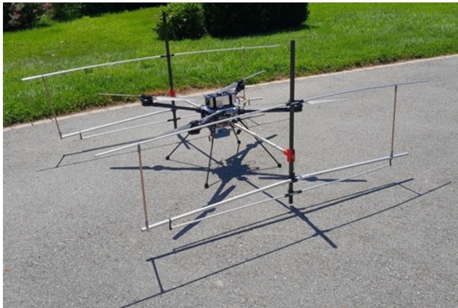
Figure 1: View of the FlyRadar instrument. The attaching mechanism (in red) between the antennas and the horizontal bar have been modified to strengthen the system.
