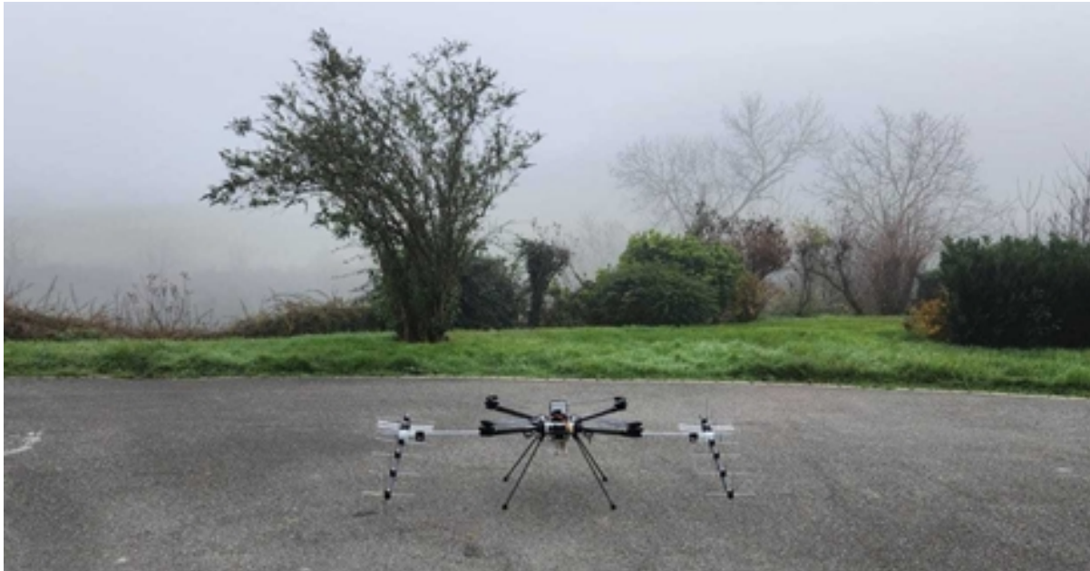
Figure 3: View of the drone with SAR antennas and a case with 3kg under the drone. Drone ready for take-off.
