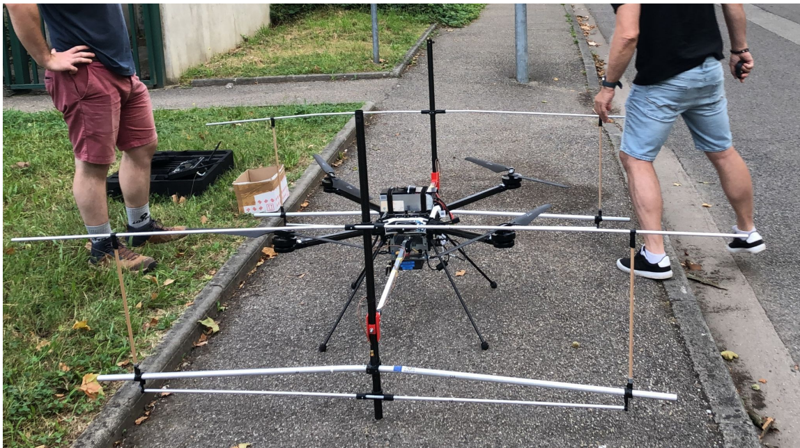
Figure 10: The complete system before the flight. The receiving rate of the control computer was found to be too low.
