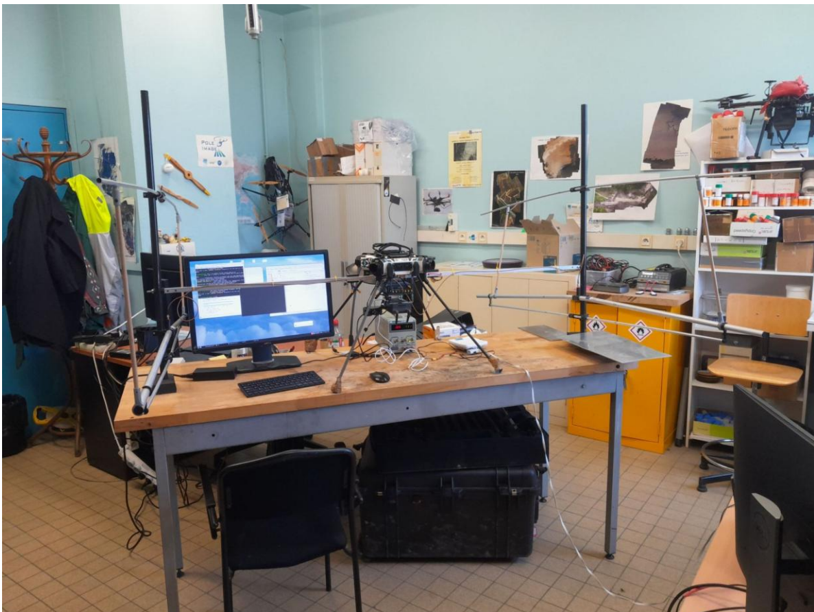
Figure 5: Test of the radar in the laboratory with the drone in “off” position. The radar is installed on board the drone. The GPR antennas are visible on both sides of the drone. The computer is connected to the radar to activate the emission and reception of the signal. In this configuration, a plate in aluminium is set under the emission antenna to test the possible interferences with the environment.
