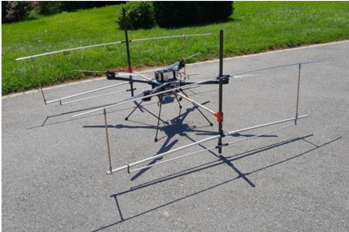
Figure 1: View of the FlyRadar instrument with the sounder antenna. The attaching mechanism (in red) between the antennas and the horizontal bar have been modified to strengthen the system.
